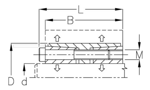
$\begin{array}{lll} \text{B mm} & = 40 \\ \text{d H8 mm} & = 28 \\ \text{D mm} & = 55 \\ \text{Fit tolerance} & = \text{Aksel h8, Nav H8} \\ \text{F kN torque} & = 35.4 \\ \text{L mm} & = 46 \\ \text{M mm} & = \text{M6} \\ \text{P N/mm2 surface pressure on shaft/hub} = 34 \\ \end{array}$
